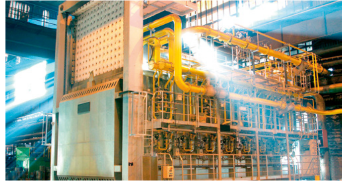
Ceramics industry: intermittent shuttle kiln
